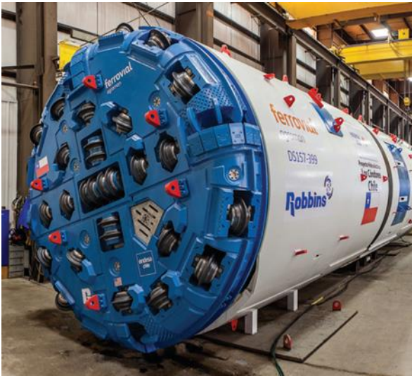
Figure F.6: Tunnel boring machine
